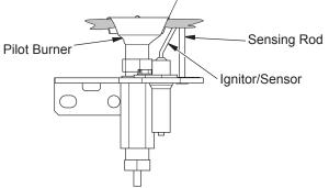
Figure 51 - Correct Pilot Flame Pattern
